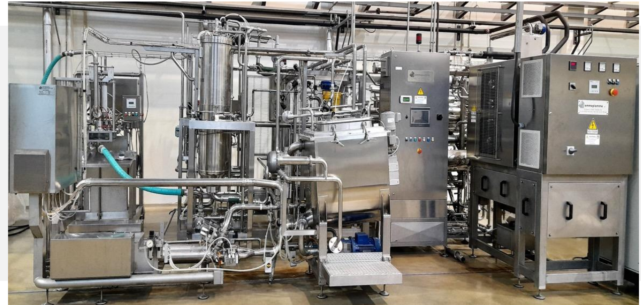
30 kW, 350 L/h Continuous Ohmic Heater – Aseptic Processing (Inovlinea, Tagusvalley, Abrantes, Portugal)
